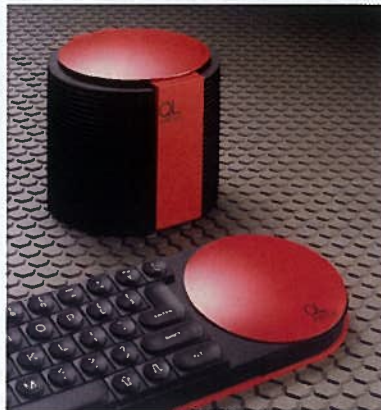
► Beyond the QL... Rick Dickinson's prototype design for the QL Plus, with built-in wafer drive and accompanying wafer stack. The design never progressed beyond this model.
